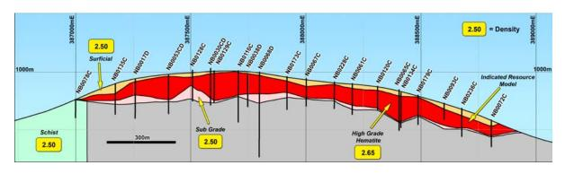
FIGURE 5: DRILLHOLE LOCATIONS AT NABEBA DEPOSIT
