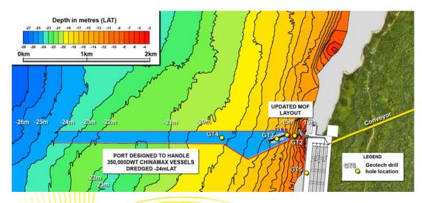
Figure 11: Port Layout for Chinamax Shipping
