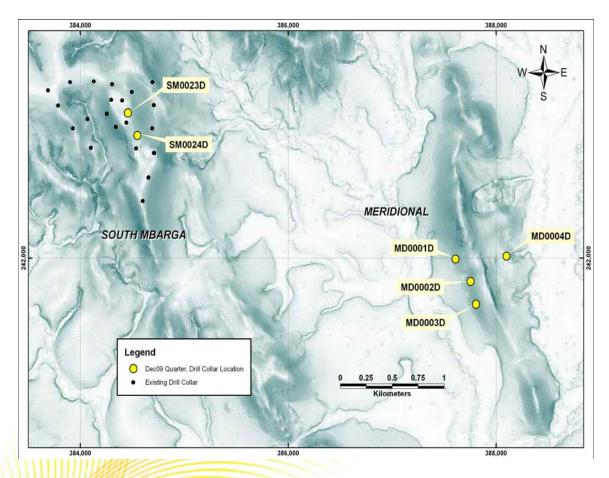
Figure 7: Location of Drill Holes completed on the Mbarga South and Meridional Deposits in December 2009
