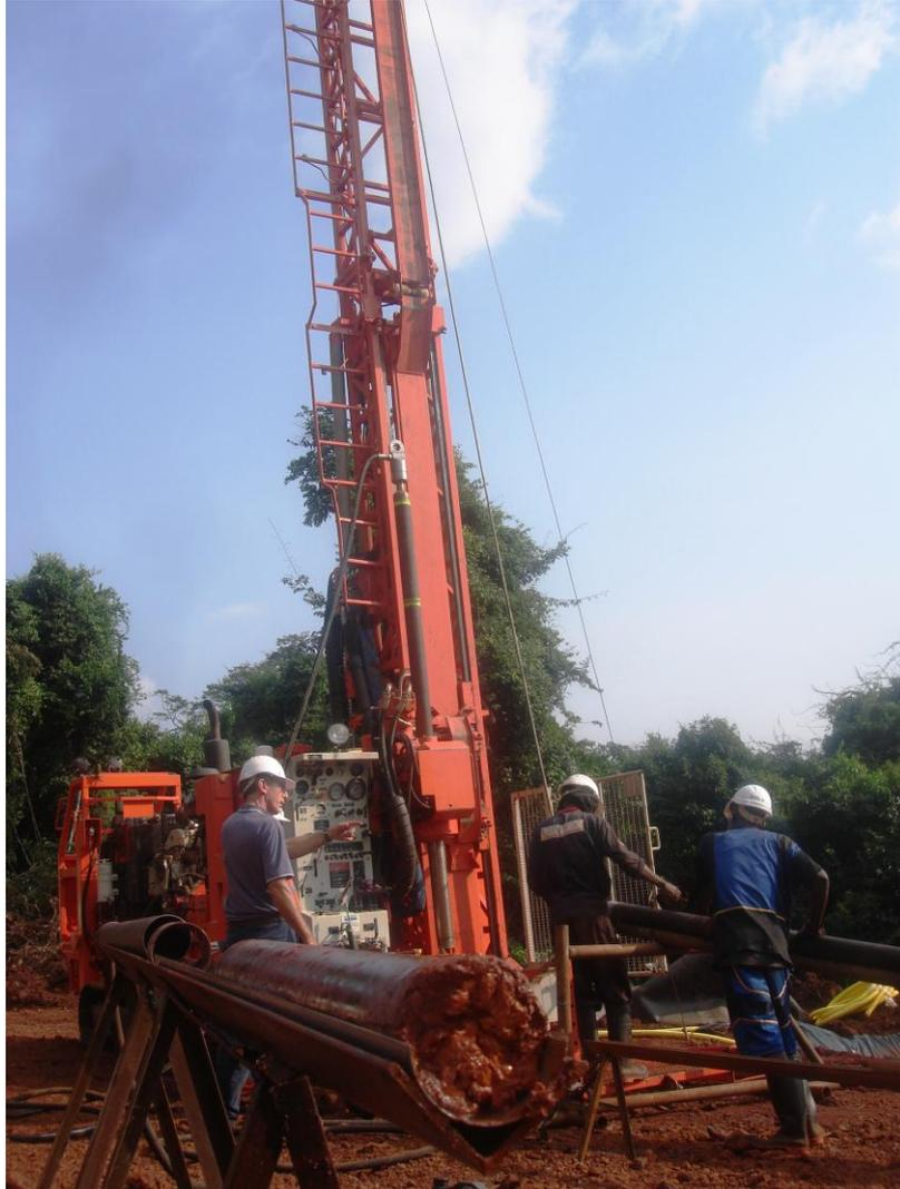
**Figure 2: Sandvik DE710 Drill Rig operating at the Nabeba Deposit**
