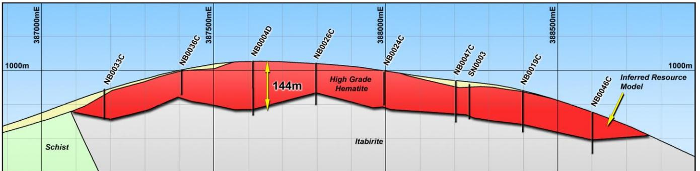
Figure 5: Oblique Section through Nabeba looking north-west showing thickness of up to 144 m of high grade hematite
