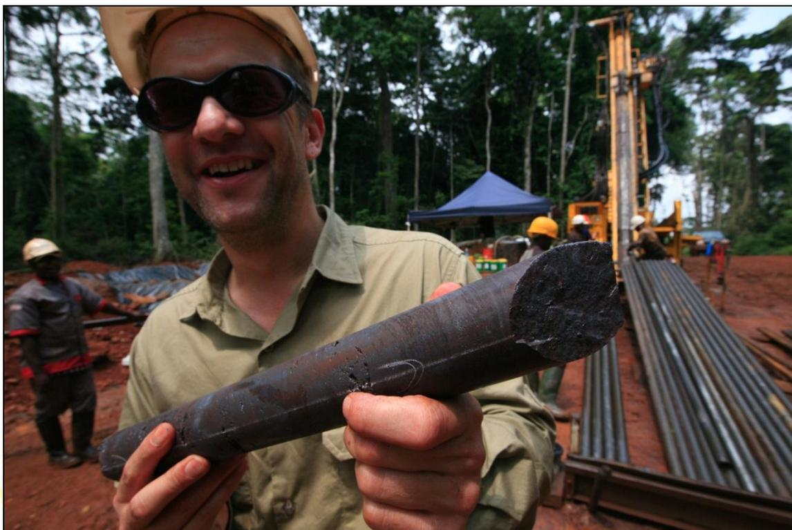
FIGURE 9 – SITE GEOLOGIST WITH MASSIVE HEMATITE DRILL CORE SAMPLE FROM DEEP 'HYPOGENE' STYLE MINERALISATION
