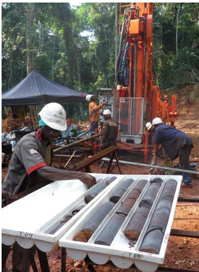
Figure 8: PQ Drill Core recovered from drilling on the Meridional Deposit in December 2009
