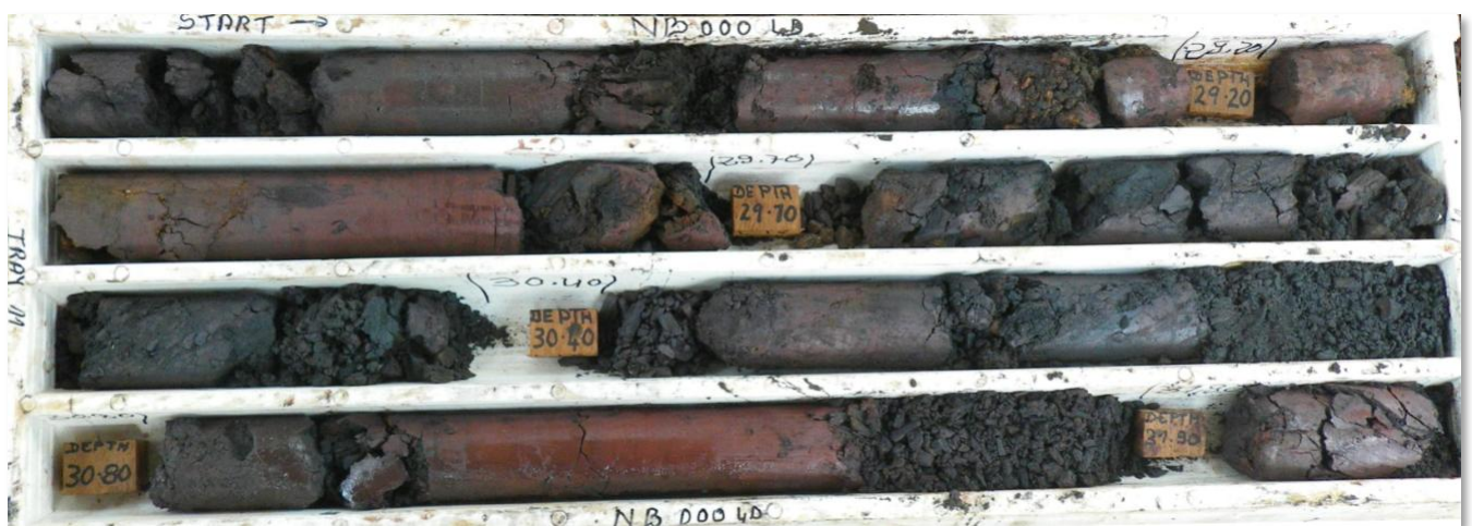
Figure 3a: Sample core photographs from Diamond Drill Hole NB0004D (from approximately 28m to 32m)
